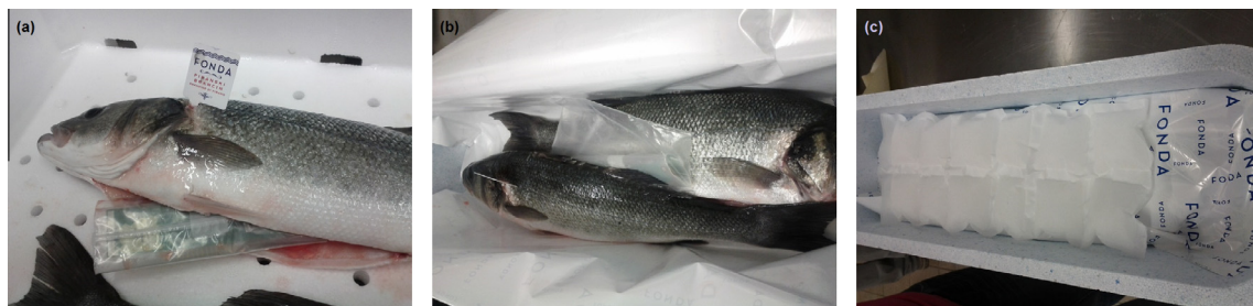
Fig. 3. Packing and monitoring temperatures (FG): in the gutted fish-TDL 1 (a); between the fish-TDL2 (b); placement of the hydrated and frozen gel pad on top of the fish in the box (c).
