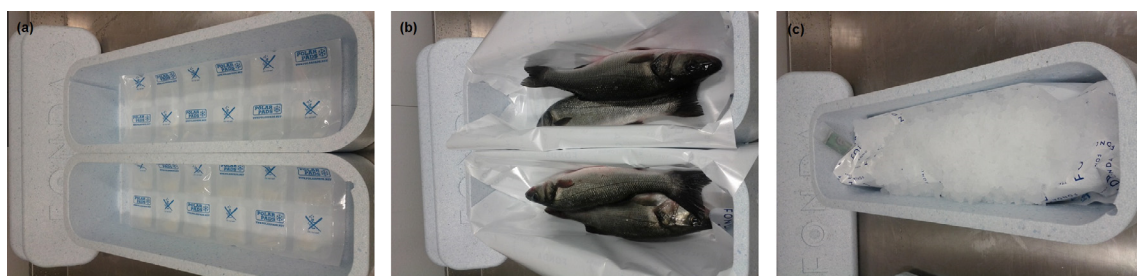
Fig. 4. Packing and monitoring temperatures (DG + WI): dry, non-hydrated gel pad on the bottom of the box (a); monitoring temperatures in the gutted fish-TDL 1 (b); monitoring temperatures in the box-TDL 2 (c).
